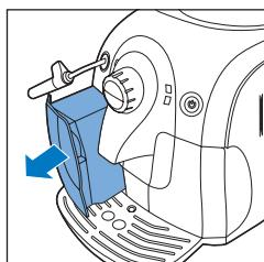
1 Remove the water tank from the machine.
