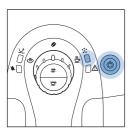
The descaling light and the on/off button light up continuously. You have to descale the machine. Follow the instructions in chapter 'Descaling the machine'.
