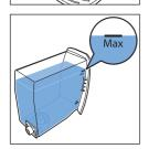
**3** Fill the water tank with cold tap water up to the MAX indication.
