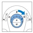
2 Turn the control dial to the hot water icon and brew hot water. Let hot water flow out of the hot water/steam wand for 10 seconds.
