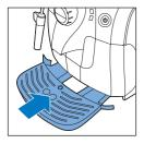
Note: Make sure the drip tray is fully inserted.
