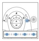
The warning light flashes slowly. The brewing unit is not correctly inserted, the coffee grounds container is not inserted, the maintenance door is open or the control dial is not in the correct position.
