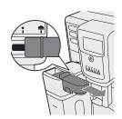
**Warning**: before selecting a milk-based coffee beverage or milk froth, ensure the milk carafe is installed and the milk dispensing spout is open. If the milk carafe is not correctly installed, the milk dispensing spout may spray steam or hot milk.
