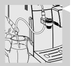
4 Insert the suction tube into the milk container.
