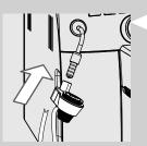
27 Insert the Automatic Milk Frother on the rubber grip until it locks into place.
