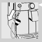
2 Remove the Automatic Milk Frother from the steam/hot water wand.
