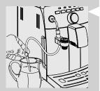
3 Insert the suction tube into the container.
