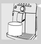
7 The steam/hot water wand ( button steady on) and the dispensing spout ( button steady on) start dispensing the descaling solution.
