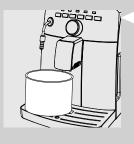
9 Empty the container and place it back under both the steam/hot water wand and the dispensing spout.
