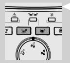
7 The machine warms up and the " and " buttons flash. The " button turns off.
