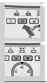
2 Press the "" button to start the cycle. The machine starts the automatic priming of the circuit by dispensing some water through the steam wand.
