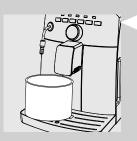
4 Place a container under the steam/hot water wand and the coffee dispensing spout.
