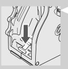
10 Gently pull down the lever until it is in contact with the brew group base and the two reference signs on the side of the brew group match.
