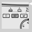
12 Start the rinse cycle by pressing the flashing U button.
