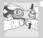
20 To detach the Automatic Milk Frother, press the sides and remove it by applying light lateral movements as shown in the figure.
